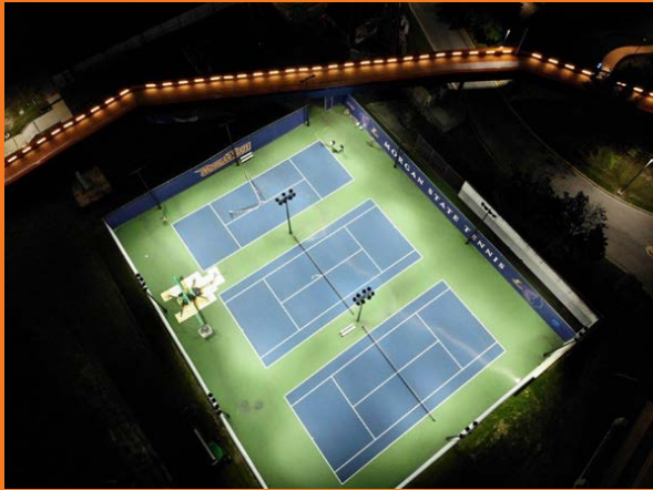
Morgan State University (126) Mledtech RT410FL-260W LED Sports Lights 80FC Average Uniformity 0.60
